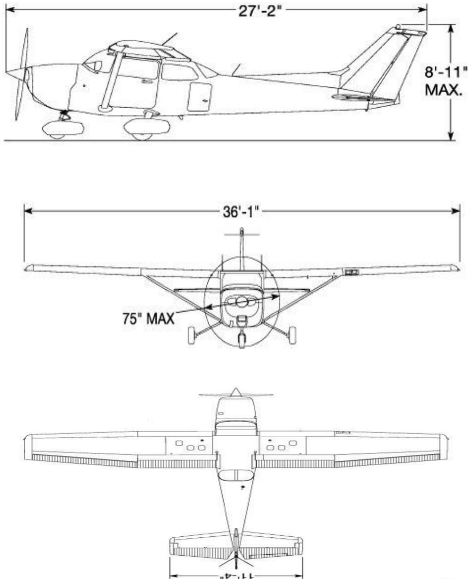
**Fig: Three view drawing-Cessna 172R aircraft**
